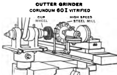
FIG. 20. — GRINDING INSERTED TOOTH MILLING CUTTER.
